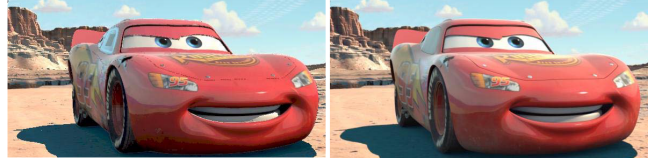
Figure 11: The left image was rendered by Lpics and the right one by a software renderer. Users need to wait for about 0.1s after moving one light to get a respond from Lpics while it takes 2000s with the software renderer [Pellacini et al. 2005].
