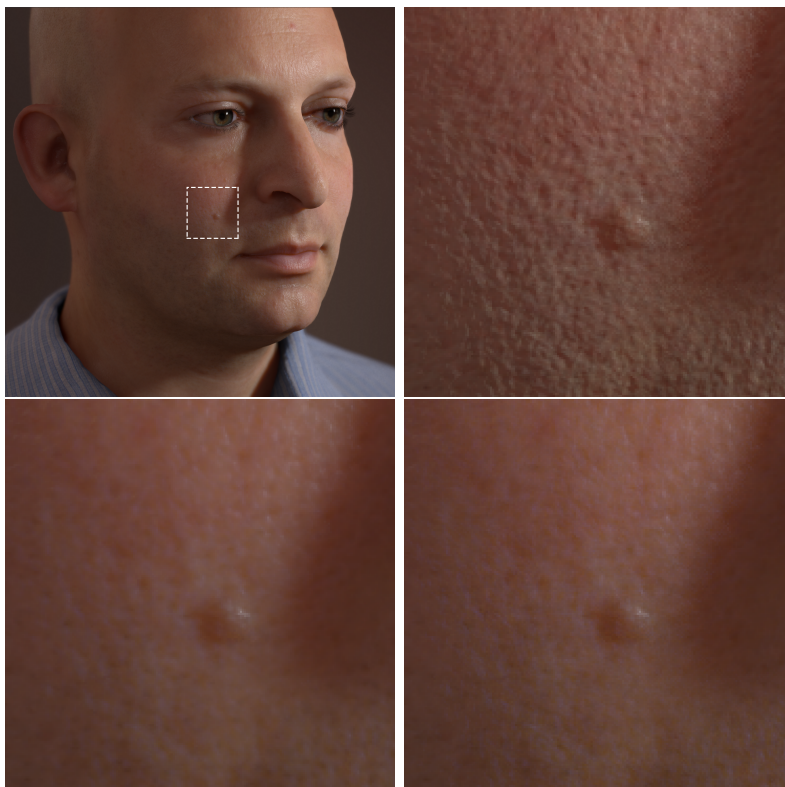
Figure 5.41: The quality of the rendered images, with and without importance sampling of the approximated kernel. (a) Initial image; (b) Uniform sampling with only seven samples leads to obvious aliasing artifacts; (c) Ground-truth created by uniform sampling with 513 samples; (d) Our importance sampling with as low as seven samples.
